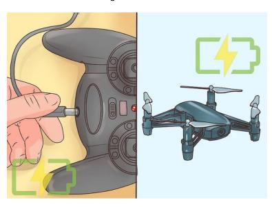
Figure 4.1. 6 Charging Remote and Drone
