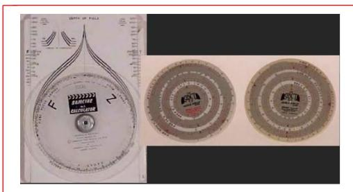
Figure 2.1. 40 Depth of Field calculator
