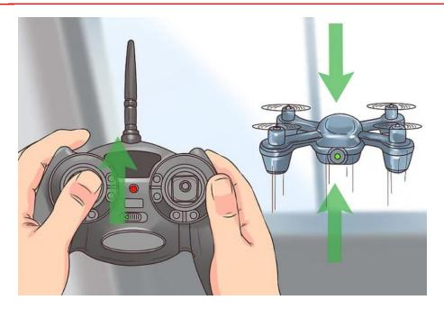
Figure 4.1. 11 Changing elevation of drone
