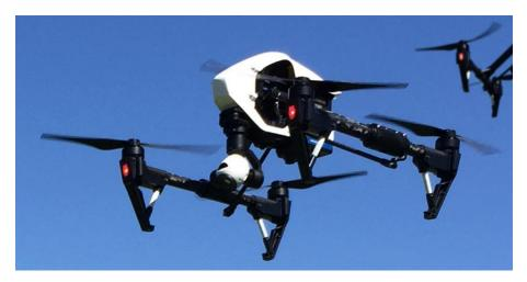
Figure 4.1. 1 Multi rotor drone
